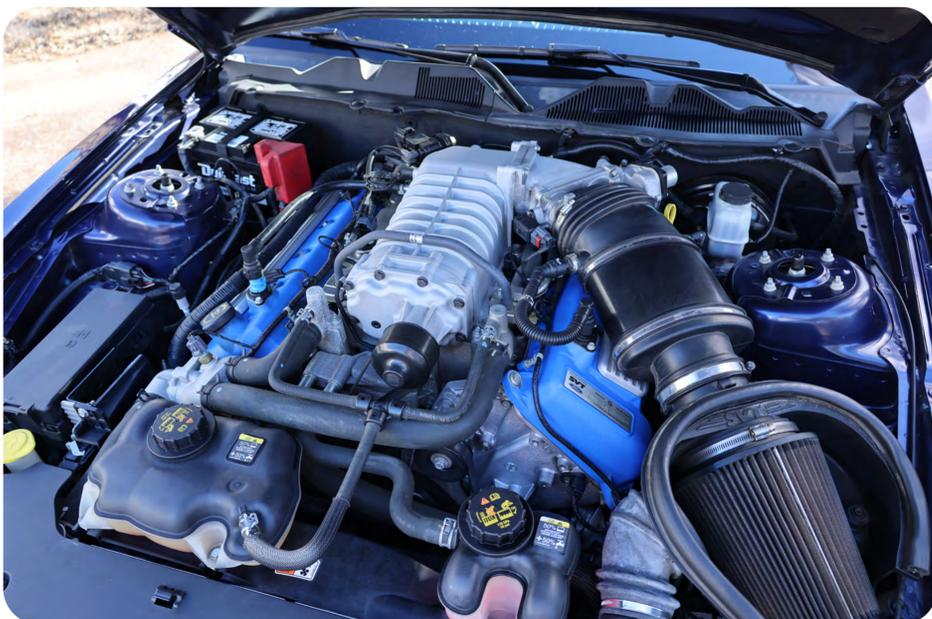
Original hand built 5.4L supercharged V8 (550hp)
