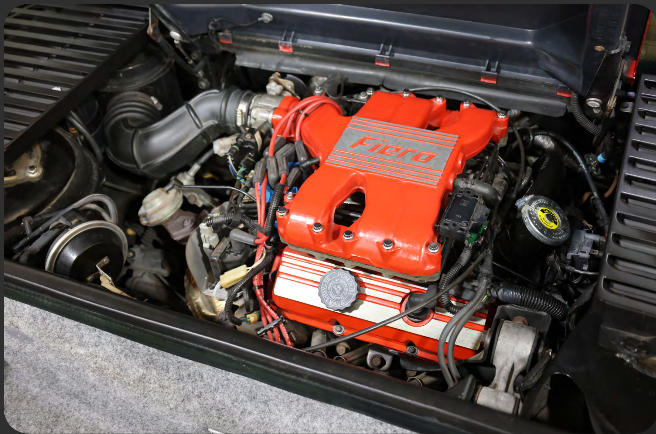
Original Multi-Port Fuel Injected (MFI) High Output 2.8L V6
